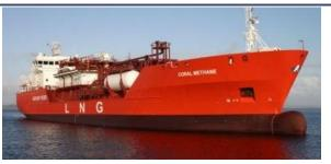
World's first combined 7,500 m<sup>3</sup> LNG/ LEG/LPG carrier
