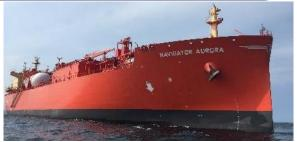
37,000 m<sup>3</sup> ethylene/ethane carrier, the largest ethylene ship in the world
