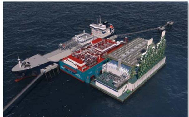
FSRUs provide a flexible solution as storage and feeding units for floating power barges. With adjustable send out rate and pressure the FSRU covers the changing demand of fuel gas on the power barge. Therefore FSRUs become an integral part of the sea based power generation and LNG-to-wire projects.
