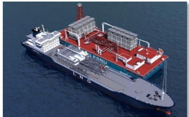
*FSRU with ambient air vaporisers and shuttle tanker*
