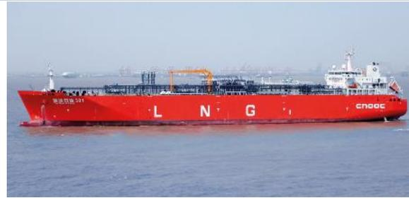
World's largest LNG carrier based on type C tanks
