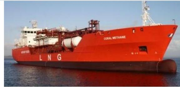
World's first combined 7,500 m<sup>3</sup> LNG/LEG/LPG carrier
